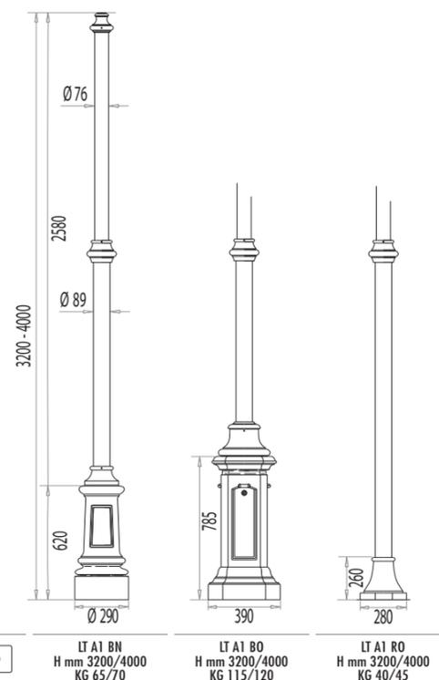
Modelli depositati | Registered design - Scala | Scale 1:30
